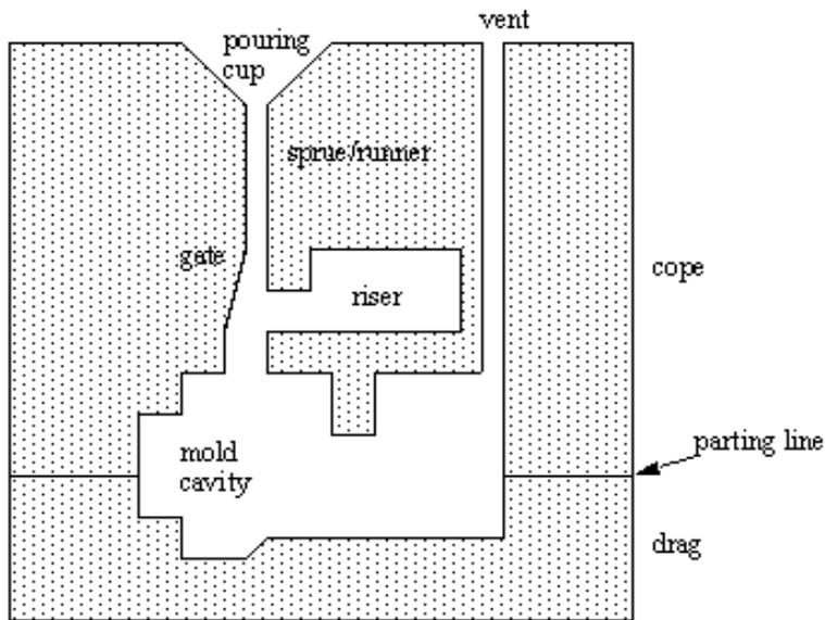
This picture shows the cross section of a sand casting mold.
