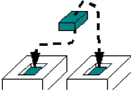
The pattern first makes an impression in the cope and drag. The impression created includes the gating system as
